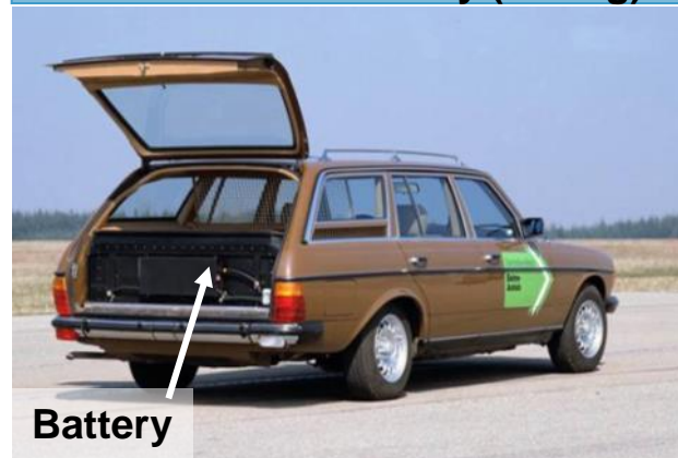
Sedan (1982) with nickel-iron-battery (600 kg) in the trunk
