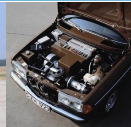
Sedan (1982) with nickel-iron-battery (600 kg) in the trunk
